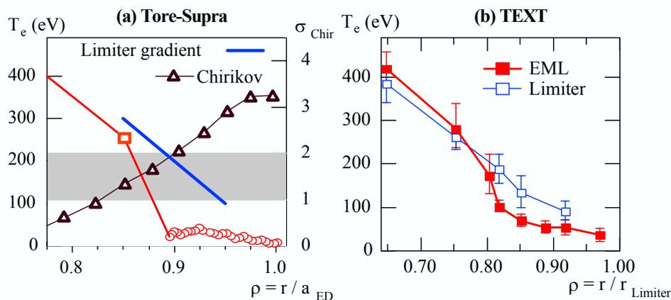
**Figure 1:** Electron temperature profiles from (a) Tore-Supra and (b) TEXT (EML=ED). In both cases the blue curve corresponds to the ED off and the red to the ED on.
