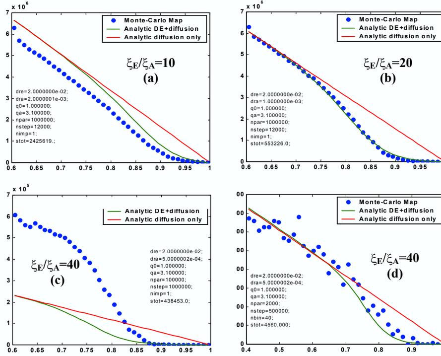
**Figure 2:** Comparisons between Monte-Carlo calculation (blue dots), analytic form with ED pinch (green) and analytic form without the pinch (red) for  $\xi_E/\xi_A = 10$  (a), 20 (b) and 40 (c and d). The latter has all toroidal correlations switched off.
