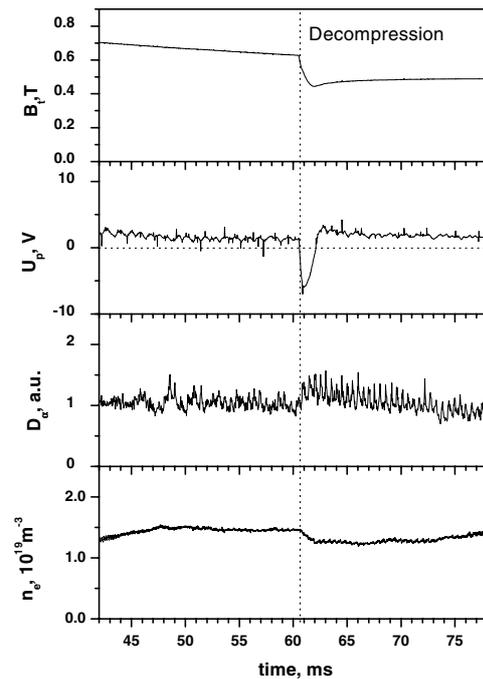
Fig.2. Waveforms of the toroidal magnetic field –  $B_t$ , loop voltage –  $U_p$ , working gas emission –  $D_\alpha$  and average electron density –  $n_e$  in a discharge with  $L$ -mode preservation during magnetic decompression,  $I_p=120$  kA.
