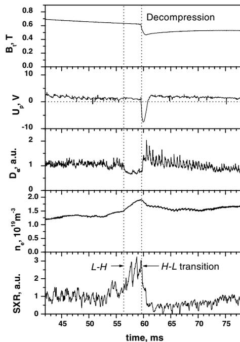
Fig.1. Waveforms of the toroidal magnetic field –  $B_t$ , loop voltage –  $U_p$ , working gas emission –  $D_\alpha$ , average electron density –  $n_e$  and soft X-ray emission – SXR in a discharge with the  $H$ - $L$  transition during magnetic decompression,  $I_p=120$  kA.
