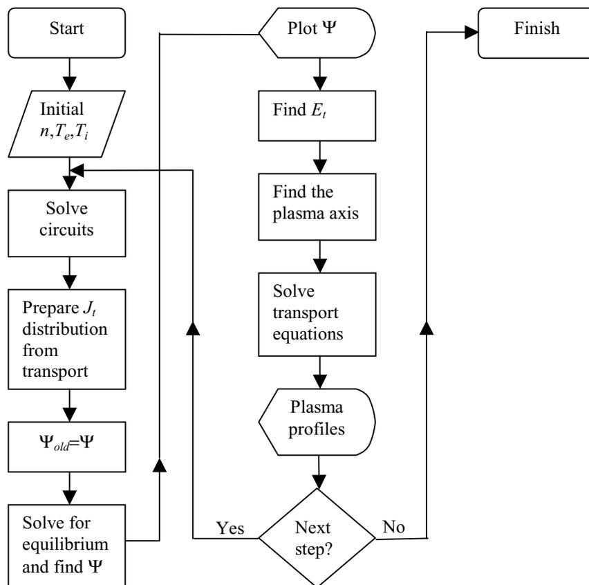
Fig. 1. Flowchart of simulation of the self-consistent plasma equilibrium and transport.
