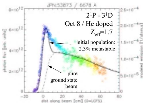
Fig 6 HeI beam emission profile of the  $2^1P-3^1D$  singlet line (He doped beam 130 keV).
