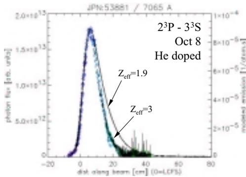
Fig. 5: HeI beam emission profile of the  $2^3P-3^3S$  triplet line (He doped beam 130 keV).
