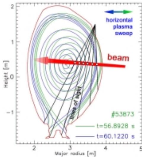
Fig. 2: Flux surfaces (EFIT) for the extreme positions of the horizontal sweep.
