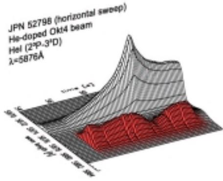
Fig.4: Beam emission profile showing the Doppler-shifted emission (right, red) and the unshifted emission (left) for a 6s doped 74 kV beam.
