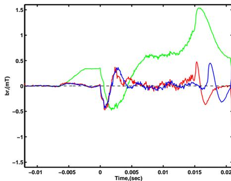
**Fig. 4.** Comparison of the experimental data and the model. Green-the sensor coil signal without feedback; blue-the sensor coil signal with feedback; red the model output. The absolute gains used for the PID controller model are:
