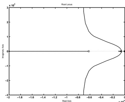
**Fig. 3.** The root locus of the feedback system. Real axis-real part of the closed loop poles,imaginary axis-imaginary part of the closed loop poles. Lines show dependence of the closed loop poles on  $g_0$ .The controller gains are:
