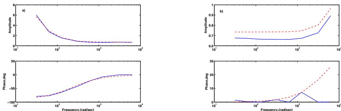
**Fig. 2.** The transfer function of the analog PID controller: a)PI controller ( $G_p = 0.75$ ,  $G_i = 0.06$ ,  $G_d = 0.0$ ), b)PD controller( $G_p = 0.75$ ,  $G_i = 0.0$ ,  $G_d = 1.0$ ). Measured (solid line) and model (dashed line) results are shown.
