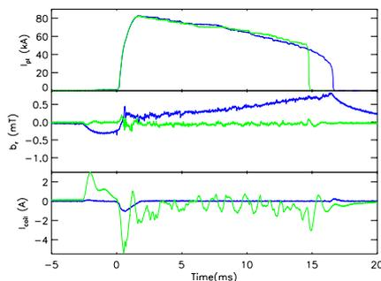
**Fig. 5.** The plasma current, the radial magnetic field and the active coil current with (green) and without (blue) feedback
