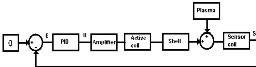
**Fig. 1.** Intelligent shell RWM feedback system in EXTRAP T2R
