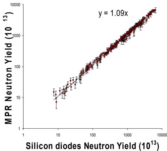
Figure 2 The pulse-integrated neutron yield data from the TTE campaign. Data from the silicon diodes are compared to MPR data.
