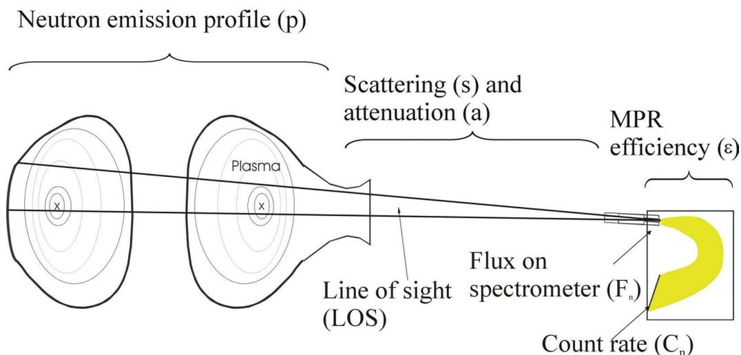
Figure 1 The components important for the determination of the JET neutron Yield.
