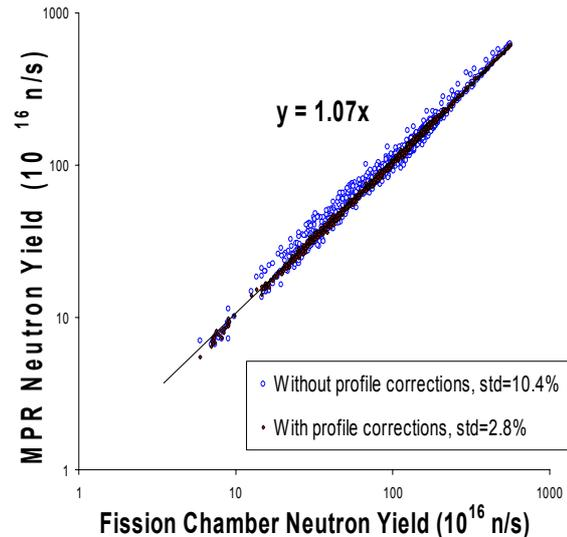
Figure 3 The 50 ms time resolved data from the DTE1 campaign. MPR data compared to fission chamber data. The importance of using profile corrections is illustrated.
