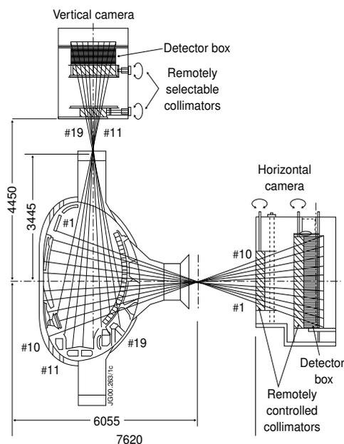
Fig. 4. Schematic view of JET neutron profile monitor
