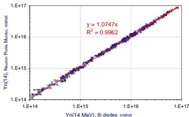
Fig.5 Comparison of 14 MeV neutron yield measured by Neutron Profile Monitor (Bicron detectors) and Si diodes (~450 TTE shots)
