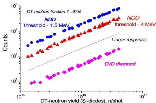
Fig. 1. NDD and CVD Diamond detectors response to Tritium JET shots ## 61084-61236
