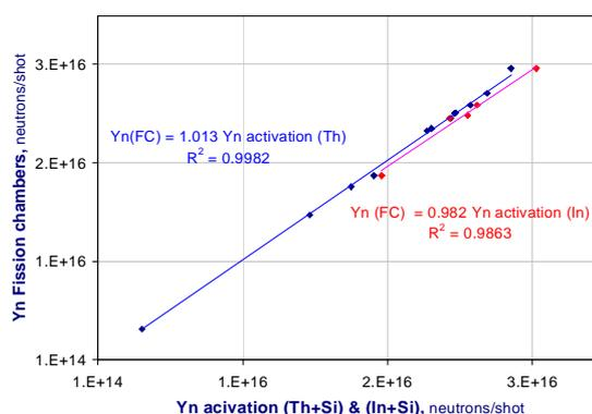
Fig. 3. Cross calibration of fission chambers against activation system for DD plasma: in red - Indium samples, in blue - Thorium samples.
