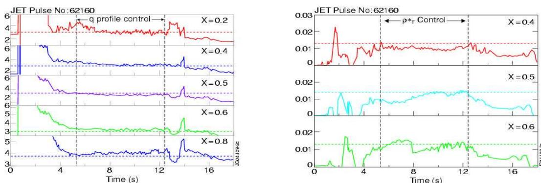
Fig1. Time evolution of the measured and requested  $q$  values (a) at 5 radii and  $\rho^*T$  values (b) at 3 radii for a controlled pulse (#62160  $B_T=3T$   $I_p=1.7MA$ , current flat top starts at 4s. Dashed lines are set point  $q$  and  $\rho^*_{Te}$  values. Control starts at 5.5s and stops at 12.3s.
