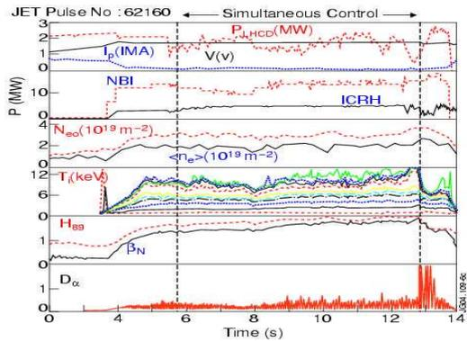
Fig2. Time evolution of the LHCD, ICRH, NBI power waveforms, loop voltage, plasma current, central and mean density, T<sub>i</sub>, H<sub>90</sub>, β<sub>N</sub>, D<sub>α</sub> of a controlled pulse (#62160, B<sub>r</sub>=3T, I<sub>p</sub>=1.7MA).
