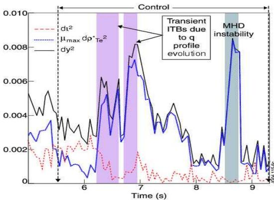
Fig6. Least square minimisation of the difference between the target i-profile (red curve) and its real time measurement (respectively the ρ\*T(x) profile (blue curve)). The sum is given by the black curve.
