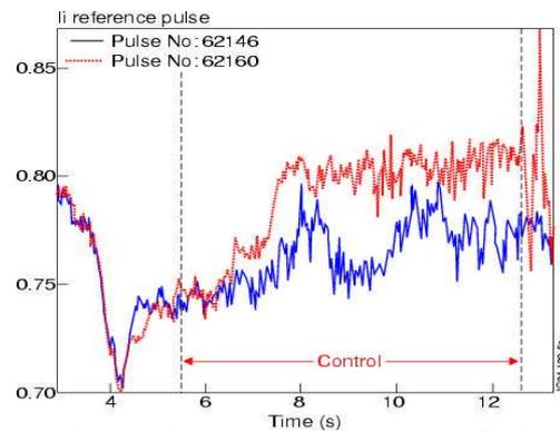
Fig3. Time evolution of the internal inductance of a feedback pulse (#62146, B<sub>r</sub>=3T, I<sub>p</sub>=1.7MA) compared to a reference pulse without feedback (#62160, B<sub>r</sub>=3T, I<sub>p</sub>=1.7MA)
