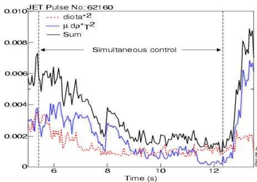
Fig4. Least square minimisation of the difference between the target i-profile (red curve) and its real time measurement (respectively the ρ\*T(x) profile (blue curve)). The sum is given by the black curve.
