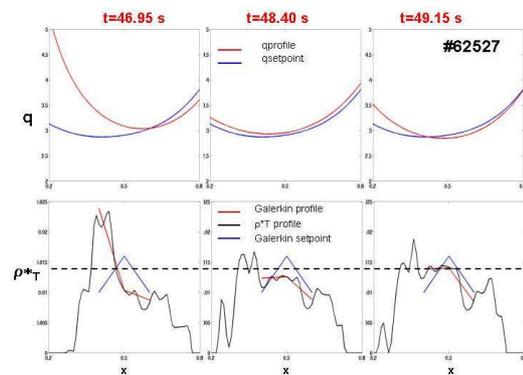
Fig5. Time evolution of measured (red) and required (blue) q- and ρ\*T profiles for a controlled pulse (#62527 B<sub>r</sub>=3T, I<sub>p</sub>=1.7MA). Control starts at 5.5s and stops at 9.15s. The black curve is the measured ρ\*T profile and the dotted line the JET criterion to get an ITB
