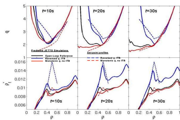
Fig7. Comparison of two closed loop simulations with JETTO for different target q and ρ\*tr profiles. The picture shows also the open loop reference simulation.
