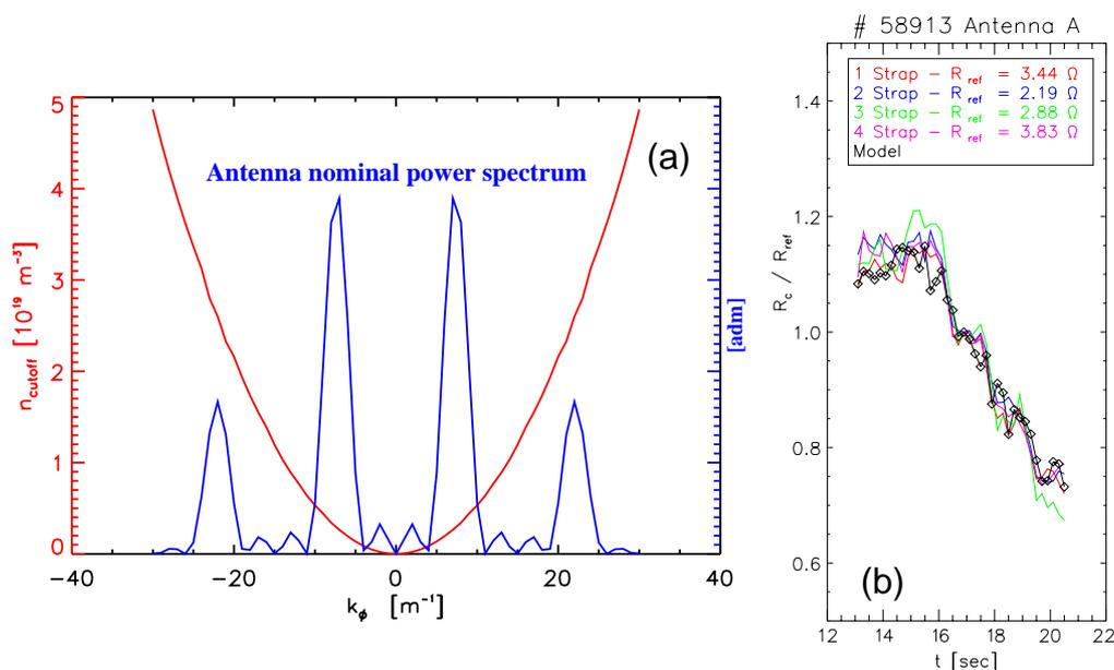
Figure 2: The frame (a) shows the cutoff density as function of the toroidal wavevector. In the same frame it is reported the normalized nominal power spectrum of the JET-A2 antennas with phasing  $[0, \pi, 0 \pi]$  and frequency  $\nu = 42$  MHz. In frame (b) the time trace of the experimental values of the relative change of  $R_c$  (DOC\_U discharge) of each of the four straps of antenna A is reported together with the prediction of the model based on eqn. (3) and (4).
