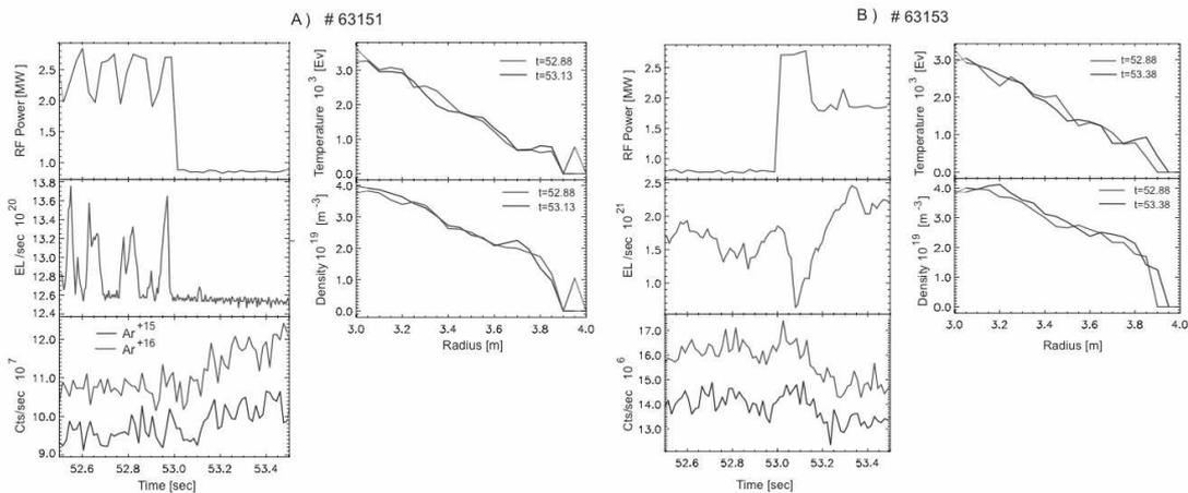
Fig. 6: A comparison of shots #63151(-pi/2) and #63153 (+pi/2): no recognizable pinch effect.
