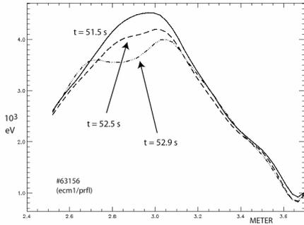
Fig. 3:  $T_e$  profile for pulse #63156 before and during RF notch
