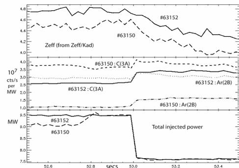
Fig. 7 : Carbon emission compared to the Ar emission for same input power but different Ar injection rates.
