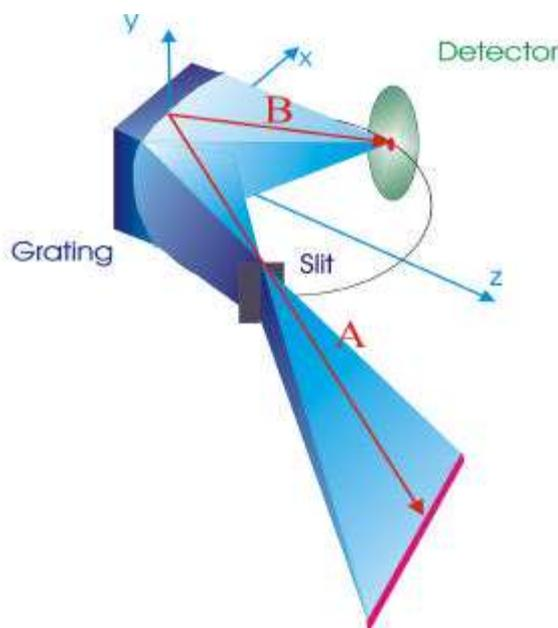
Fig.1 Image creation by spherical grating based spectrograph. The thin layer of emission source, which is located in vertical focus of the device, is imagined as a point in a detection plane.
