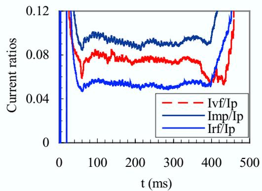
Fig.8 Current ratios of shaped field coils with power supply in series for shot 1573
