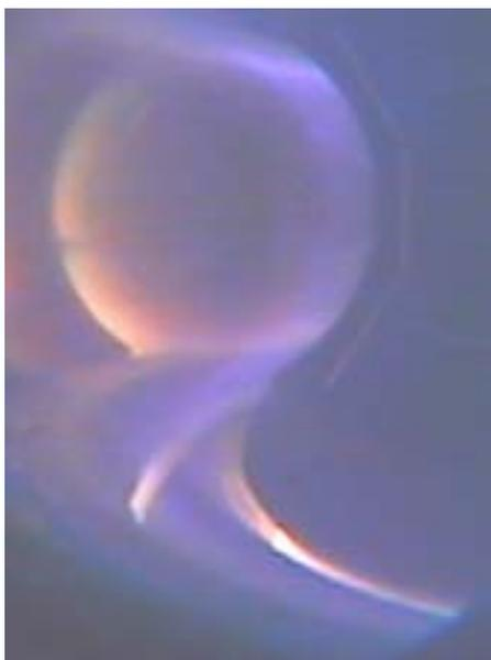
Fig.4 Divertor discharge photography at about 200 ms for shot 1766
