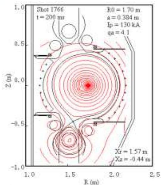
Fig.5 Reconstruction of magnetic surface from 18 Mirnov signals for shot 1766
