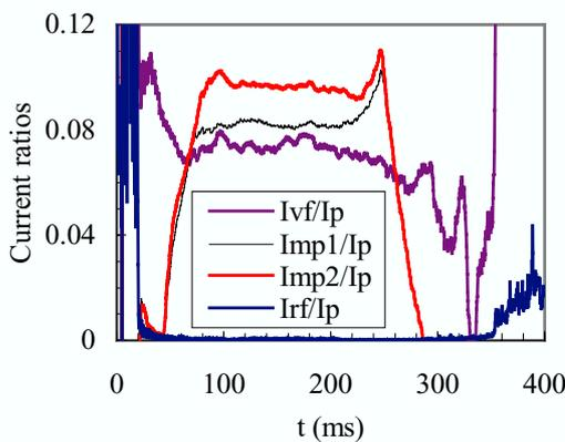
Fig.7 Current ratios of shaped field coils with bypass power supply for shot 1766
