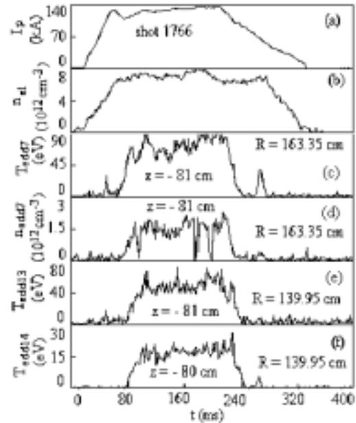
Fig.6 Parameter evolution of divertor discharge for shot 1766
