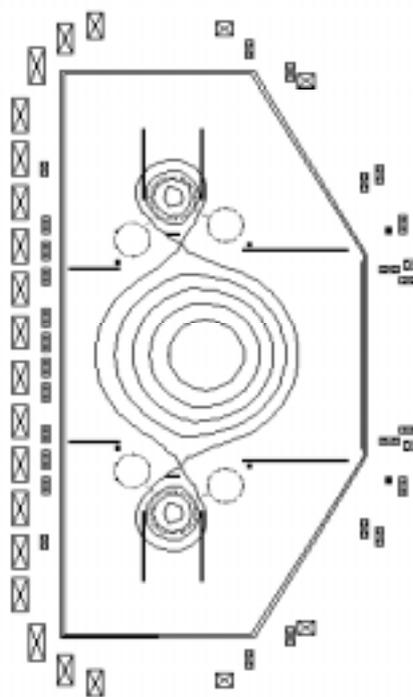
Fig.2 Double null divertor configuration simulated by SWEQU code
