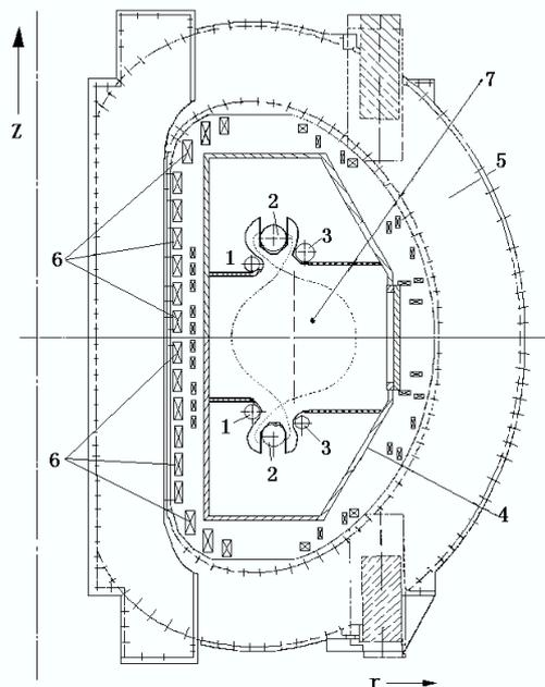
Fig. 1 Cross-section of HL-2A tokamak
