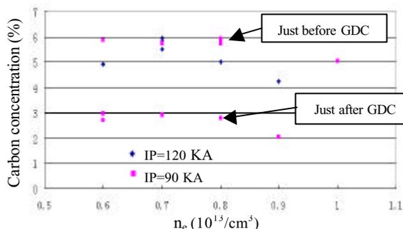
Fig.3. Carbon concentration vs. electron density
