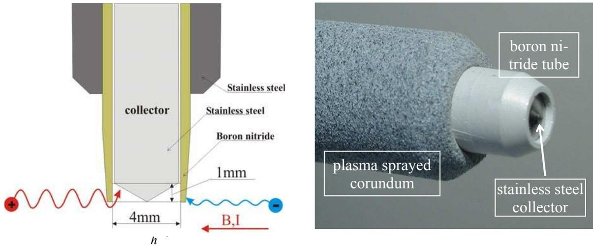
Fig. 1. Schematic and photograph of the ball-pen probe.
