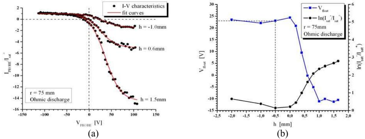
Fig. 2. (a) I-V characteristics for various collector positions.  $h$  is negative when the collector is inside the shielding tube; (b) floating potential  $V_{fl}$  and  $\ln(R)$  with respect to  $h$ . The radial position of the probe head is at 75 mm.
