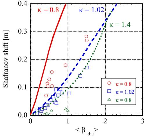
Figure. 2 Comparison the Shafranov shift measured (symbols) with theoretical prediction (lines) calculated by VMEC code for the plasma with different ellipticity of  $\kappa = 0.8, 1.02$  and  $1.4$ .
