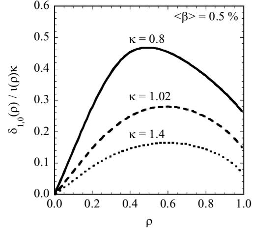
Figure. 3 Radial profiles of  $\delta_{1,0}/\iota(\rho)\kappa$  for plasma with different magnetic elongated configurations,  $\kappa=0.8, 1.02$  and  $1.4$ .
