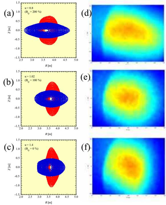
Fig. 1 (a)-(c) cross-sections of vacuum magnetic flux horizontally and vertically elongated calculated with the VMEC Code for the prolate and oblate configurations with  $\kappa = 0.8, 1.02$  and  $1.4$ . (d)-(f) tangential images of soft x-ray intensity measured with the soft x-ray CCD camera for three configurations.
