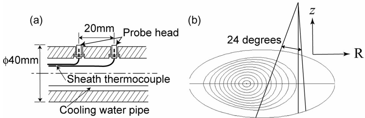
Figure 1. (a) Schematic of hybrid probe. (b) Cross-section of CHS plasma at  $R_{ax}=0.921m$  and scannable area by the two-dimensional probe drive.
