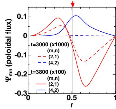
Fig.4. Profiles of perturbed poloidal flux. Red arrow indicates the position of  $q = 1/2$ .
