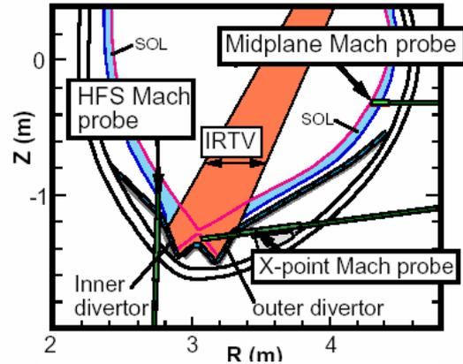
**Fig 1.** Plasma cross-section and location of reciprocating probe in JT-60U.
