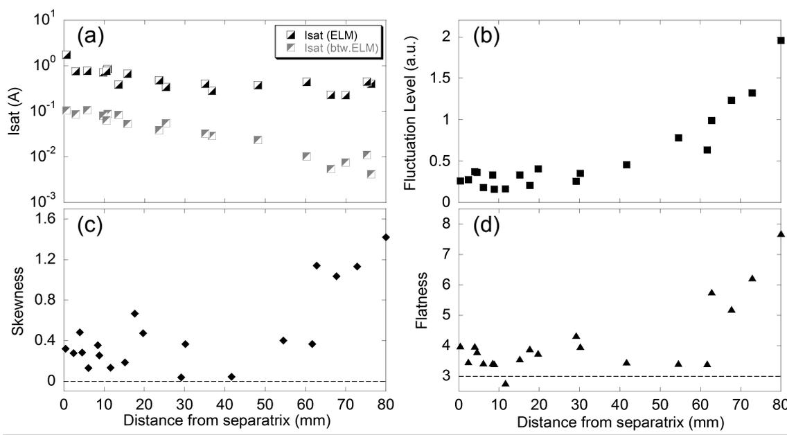
**Fig 3.** Radial profiles of (a):the peak amplitude of ELM and averaged ion saturation current of  $I_{sat}$  between ELMs, (b) normalized fluctuation level of  $I_{sat}$  between ELMs, (c)skewness and (d)flatness.
