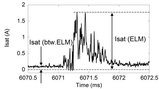
**Fig 2.** Typical time evolution of ion saturation currents measured with the mid-plane probe.
