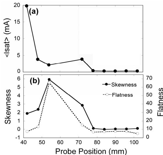
**Fig 4.** Radial Profiles of (a): averaged ion saturation current measured by the divertor probe array, (b): skewness and flatness.
