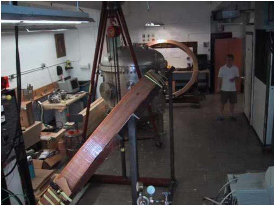
Figure 1. The poloidal field coils and the vacuum chamber in the CNT lab.
