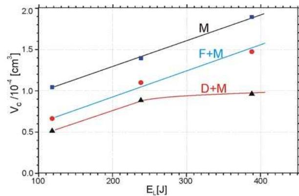
**Fig. 1:** Diagrams of the crater volumes as a function of the laser energy for different types of the targets, where: M - single target, F+M - double target with foil, and D+M - double target with disk.
