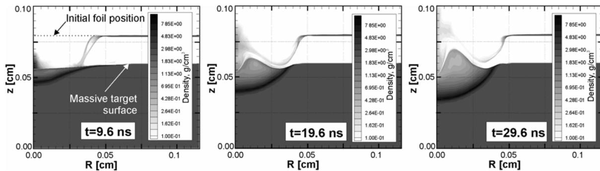
Fig. 4: Simulation of the crater formation process.
