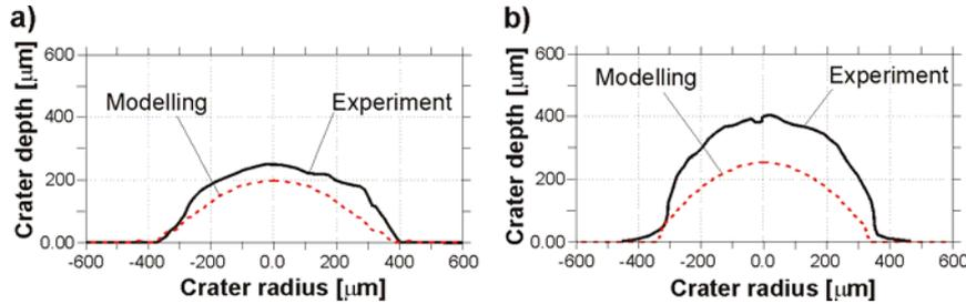
**Fig. 2:** Comparison of crater shapes and dimensions measured experimentally and calculated numerically in the case of a) double-target and b) massive target.
