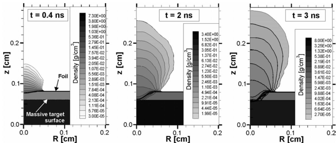
**Fig. 3:** Simulation of the ablative plasma generation and the foil acceleration.
