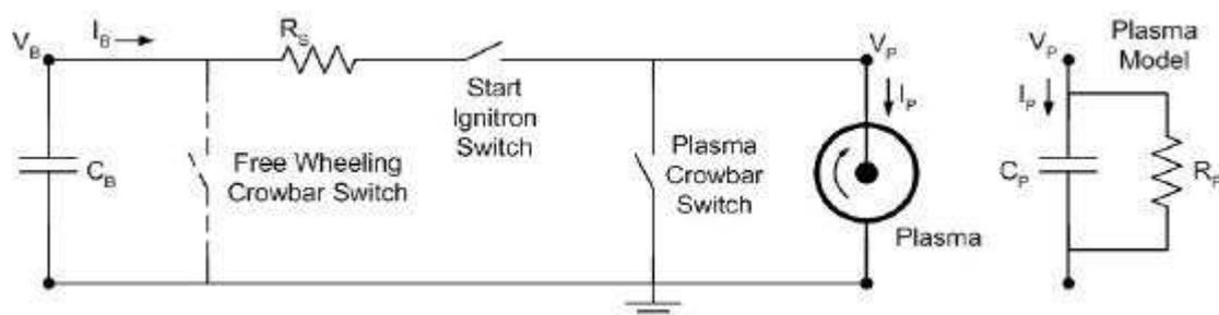
Fig 2. MCX capacitor bank.  $V_B = 5-11\text{kV}$ ,  $C_B = 1.3-7\text{ mF}$ ,  $R_S = 0.5-3\ \Omega$
