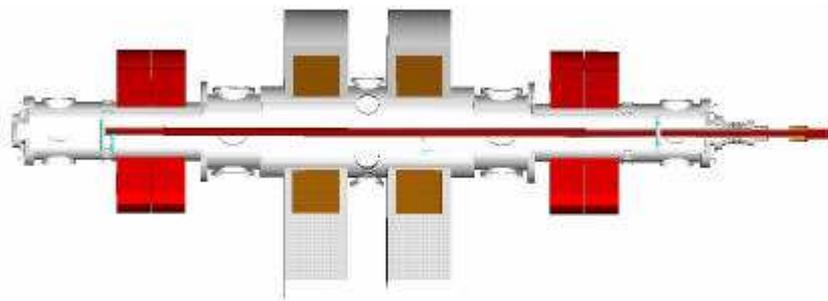
Fig 1. Cutaway of the MCX device. For scale the mirror end coils are 1m in diameter.
