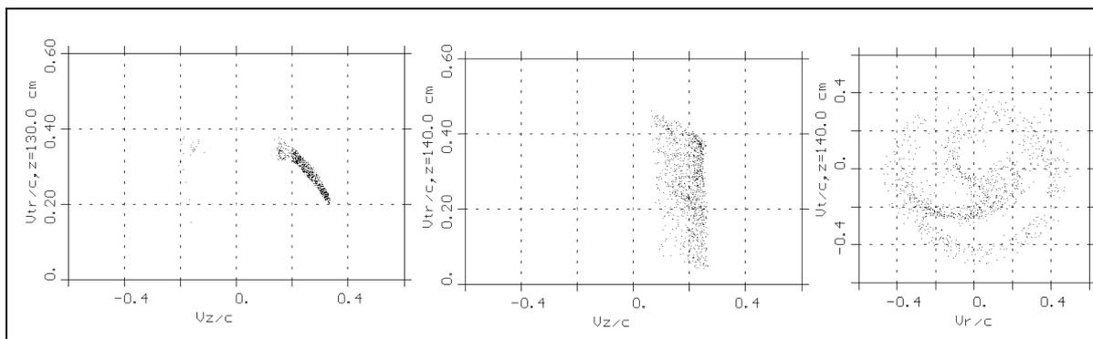
Figure 3: Evolution of the electron velocity phasespace ( $v_{tr(ansverse)}$  against  $v_{z(axial)}$  and  $v_{t(heta)}$  against  $v_{r(adial)}$ ) as the horseshoe distribution interacts with the RF wave after 40ns
