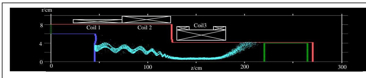
Figure 1: Configuration of the experiment as described in KARAT, colour scheme, anode:red, cathode:blue, magnets:white, RF absorber:green, macro-electrons:cyan
