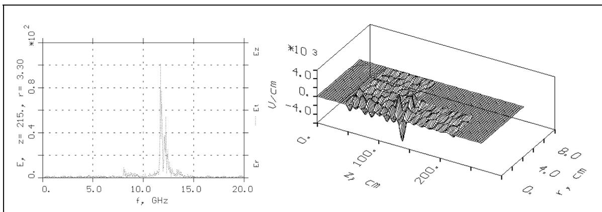
Figure 4: Spectrum of RF emissions from the electron beam and plot of the theta component of the electric field showing the excitation of the near cut-off  $TE_{0,3}$  mode after 50ns
