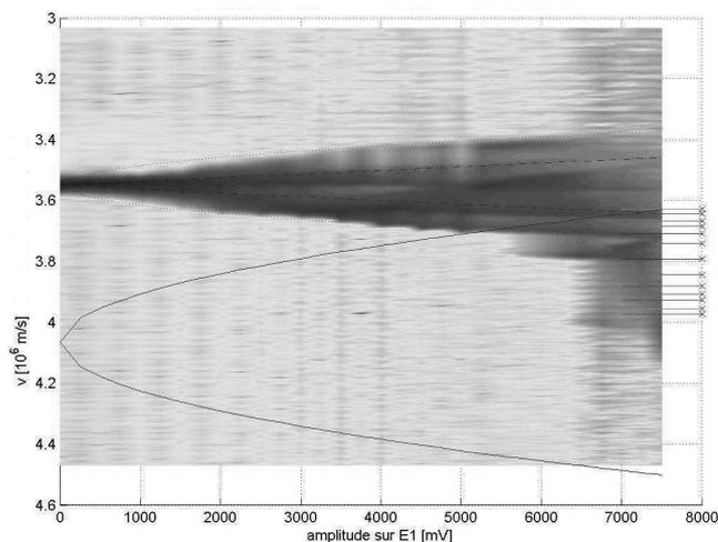
Figure 4 : Transition to chaos by overlap of beam and helix modes at 30 MHz.
