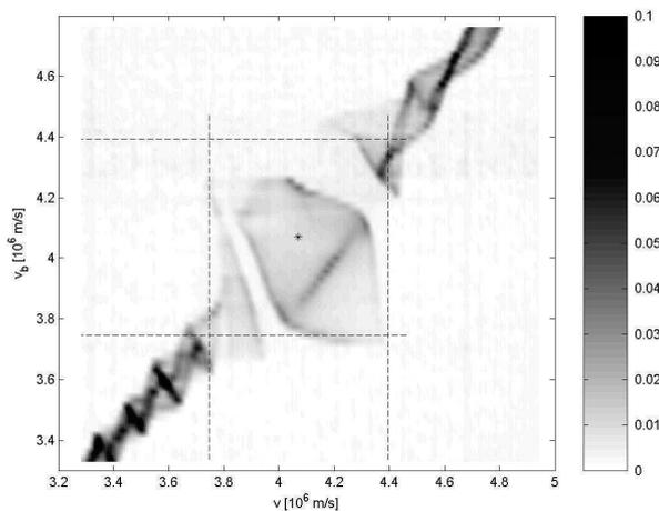
**Figure 2 :** Measured resonant velocity domain for a single wave at 30 MHz
