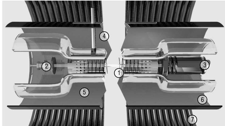
**Figure 1:** Rendering of the Travelling Wave Tube: (1) helix, (2) electron gun, (3) trochoidal analyzer, (4) antenna, (5) glass vacuum tube, (6) slotted rf ground cylinder, and (7) magnetic coil.
