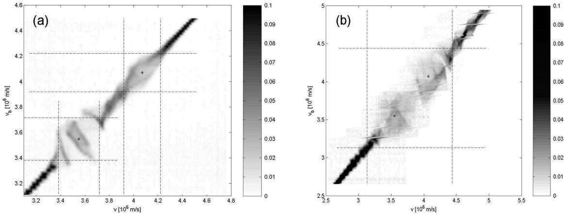
Figure 3 : Measured resonant velocity domain for two waves at 30 MHz and 40 MHz : a)  $s = 0.63$ , b)  $s = 1.5$
