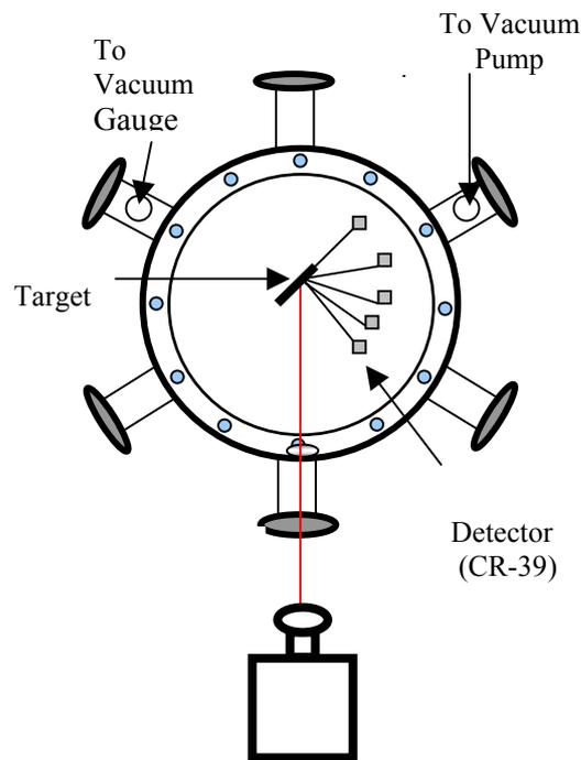
**Figure 1: A schematic of the Experimental arrangement**
