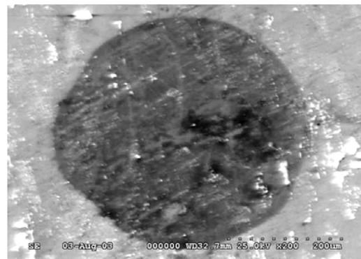
**Figure 3: SEM Micrograph of Al surface at magnification  $\times 200$  of the circular region of radius  $230 \mu\text{m}$ , circular damage is a**
