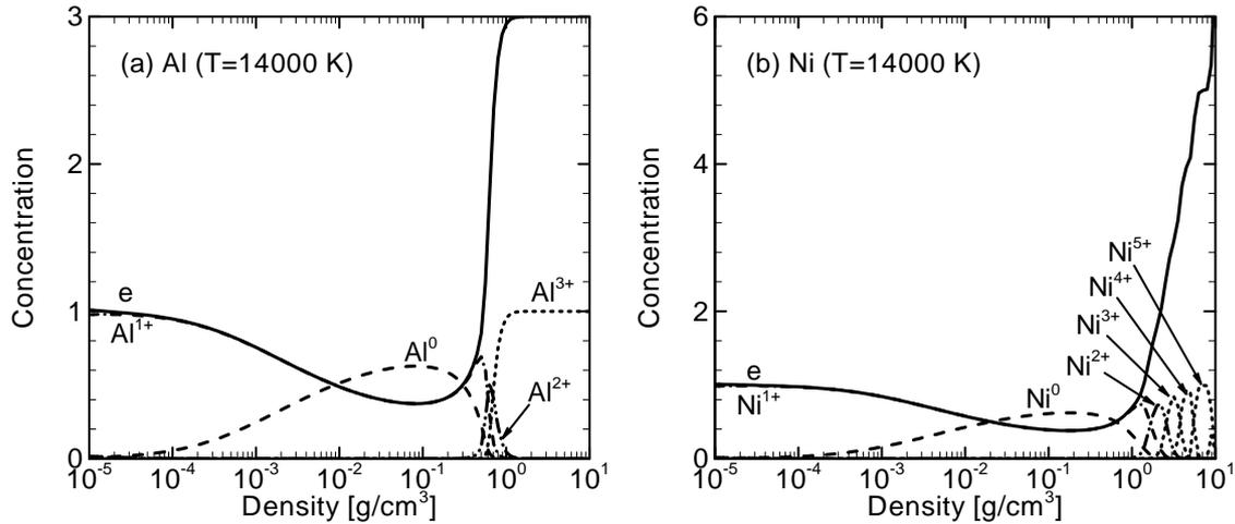
Fig. 1 Compositions of electrons, ions, and neutral atoms in warm metal plasmas computed by the present model as a function of density at  $T = 14\,000$  K: (a) aluminum and (b) nickel.
