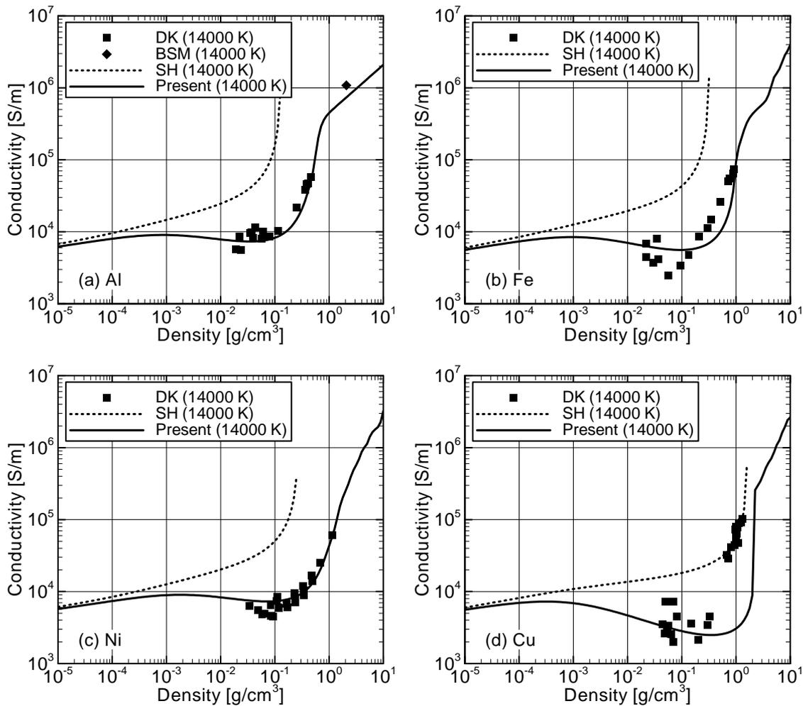
Fig. 2 Electrical conductivities of warm metal plasmas computed by the present model for (a) aluminum, (b) iron, (c) nickel, and (d) copper in comparison with the Spitzer-Härm (SH) model and the experimental data measured by DeSilva and Karsouros (DK) and Benage, Shanahan, and Murillo (BSM) at  $T = 14\,000$  K.
