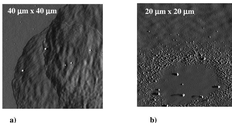
a) **Figure 3.** Craters ablated in PMMA by unfiltered pulses of 21.2-nm laser
