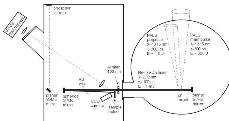
**Figure 1.** Top-view scheme of PALS vacuum chambers: Ne-like Zn laser was operated in spherical (right) chamber; ablation experiments were conducted in cylindrical (left)
