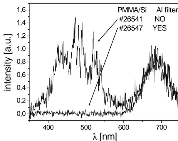
Figure 4. UV-VIS spectra emitted from PMMA surface irradiated by intense 21.2-nm radiation.
