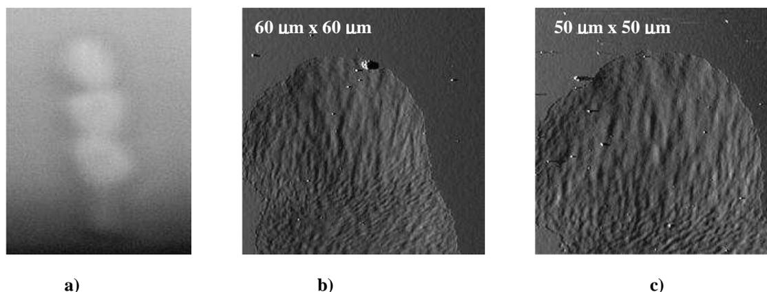
a) **Figure 2.** PMMA ablated by single pulse of 21.2-nm laser filtered by 400-nm Al foil
