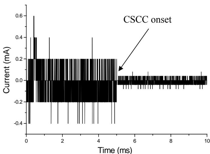
Fig. 4: The decreasing of the current fluctuations at the onset of the CSCC
