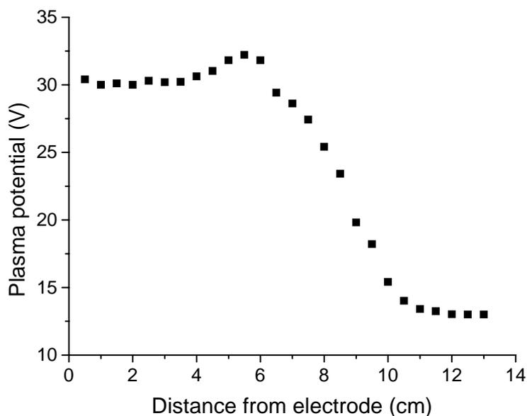
Fig. 3: Radial profile of the plasma potential in front of the electrode E after the appearance of the CSCC. Similar decreasing was recorded also for the fluctuations level of the plasma potential.
