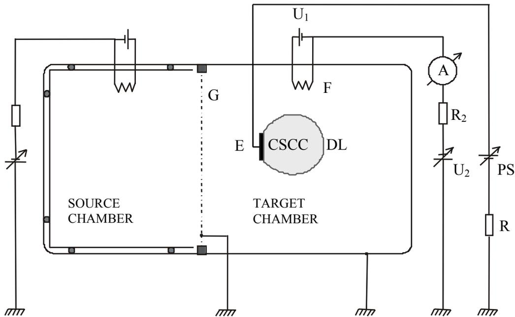
Fig. 1: Schematic of the Innsbruck DP machine. G – grid, F – filaments, E – electrode, PS – power supply, R – load resistor
