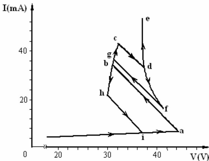
Fig. 2: Static upward and downward characteristic of the electrode E
