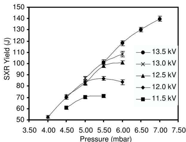
Fig. 3: Soft X-ray production for the optimised anode geometry for various operating conditions.
