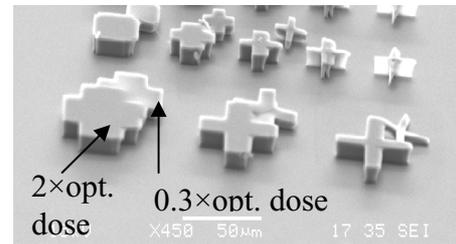
Fig. 5: Microolithography test structures on SU-8 resist.
