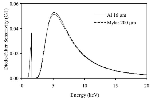
Fig. 1: Sensitivity curves for the diode-filter system.
