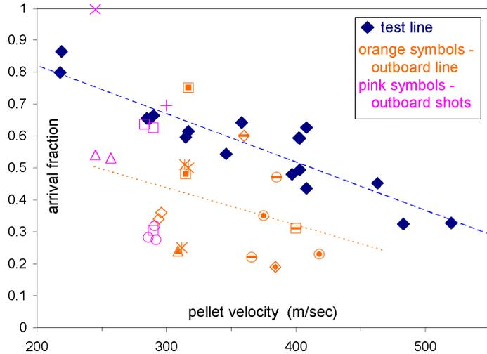
Fig.2 Fraction of pellet mass arriving at end of test line, as a function of velocity (blue diamonds). Also superimposed: equivalent data along outboard flight-line (orange), plus some of outboard pulses in text (pink) – each different symbol represents an individual shot.
