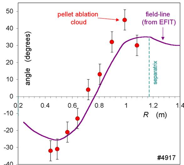
Fig.6 Measured orientation of ablation cloud for outboard injection compared with field-line angle from EFIT.
