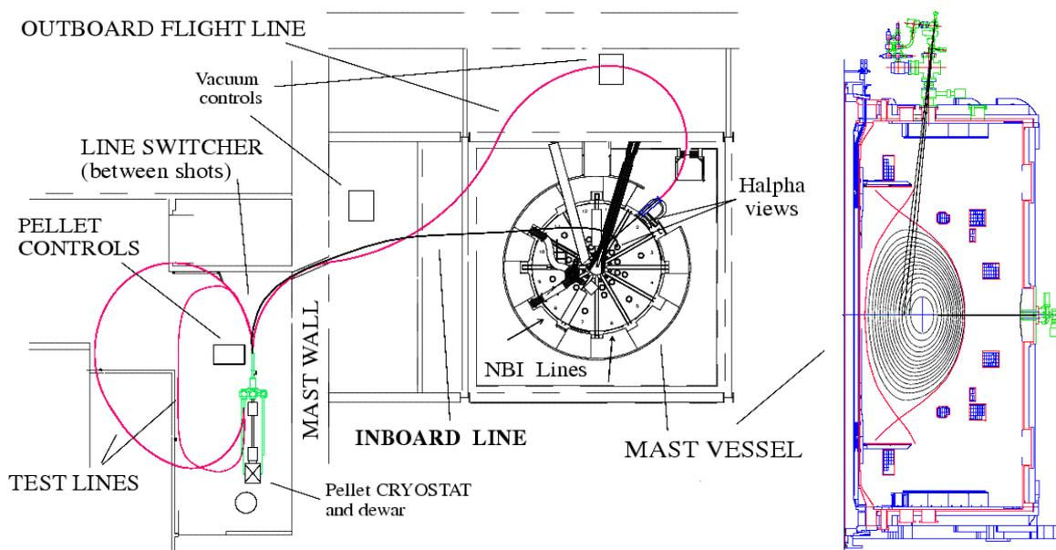
Fig.1 Top view (left) of inboard and outboard pellet tracks on MAST, plus side projection (right) of corresponding trajectories into a typical double-null plasma.
