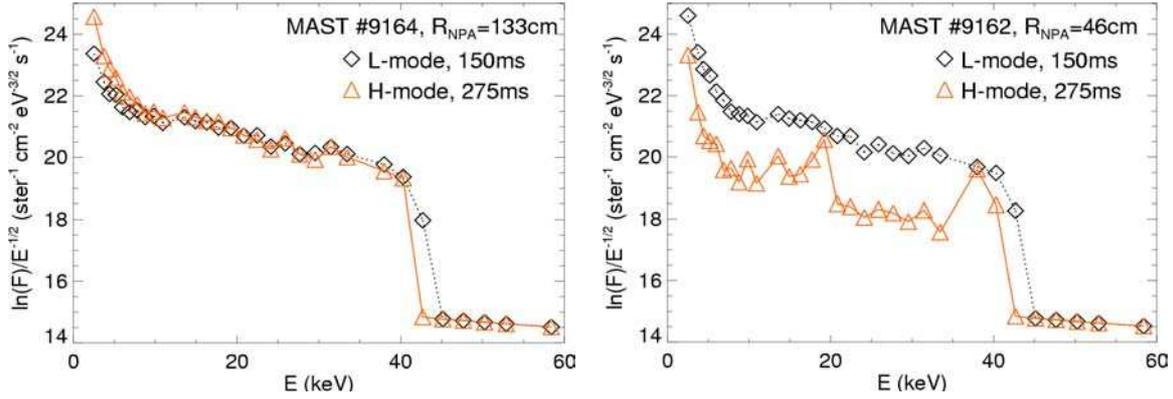
Fig. 2. The NPA spectra obtained during L- and H-mode parts of the discharge
