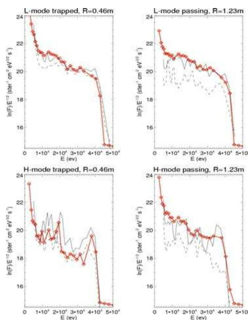
Fig. 4 TRANSP simulation of the NPA flux measurements is in agreement with experiment (diamonds).
