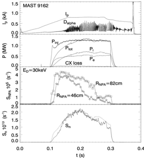
Fig. 3. TRANSP simulations of neutron yield and powers transmitted from fast ions to plasma
