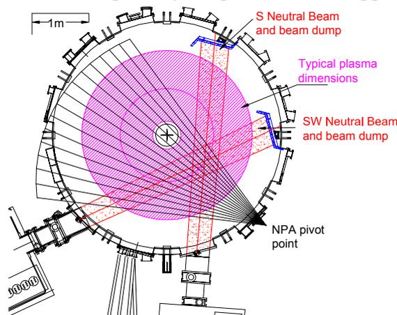
Fig. 1. MAST NBI and NPA layout.
