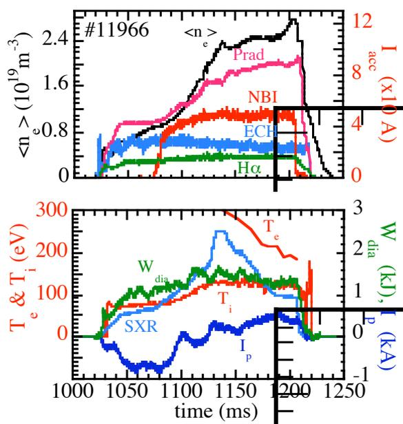
Figure 4: Time evolution of a NBI+ECH off-axis plasma discharge.
