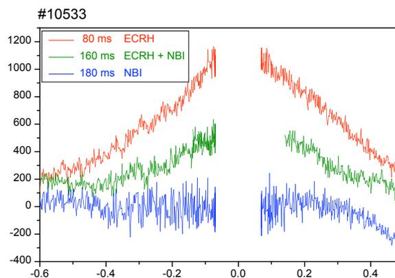
Fig 3: Profiles of plasma potential (V) by HIBP
