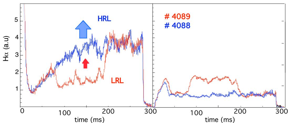
**Fig. 1.**  $H\alpha$  signals for two consecutive shots at two toroidal positions. In blue is depicted a shot with high ripple losses (HRL) during all the discharge. In red, a shot with a transition to a low ripple losses (LRL) regime.
