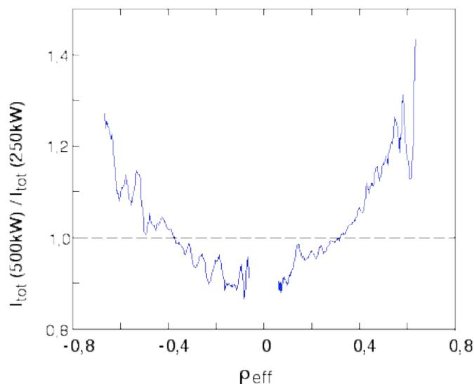
**Fig. 4.** Ratio of secondary Cs<sup>++</sup> ion current for the two different input power of Fig 3.
