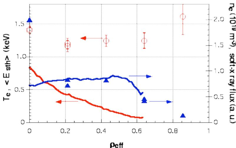
**Fig. 2.** Radial profiles of Thomson  $T_e$  (red line) and  $n_e$  (blue line) and suprathermal mean energy (open circles). Blue triangles are the measured Bremsstrahlung intensity in the energy range between 4 and 10 keV.
