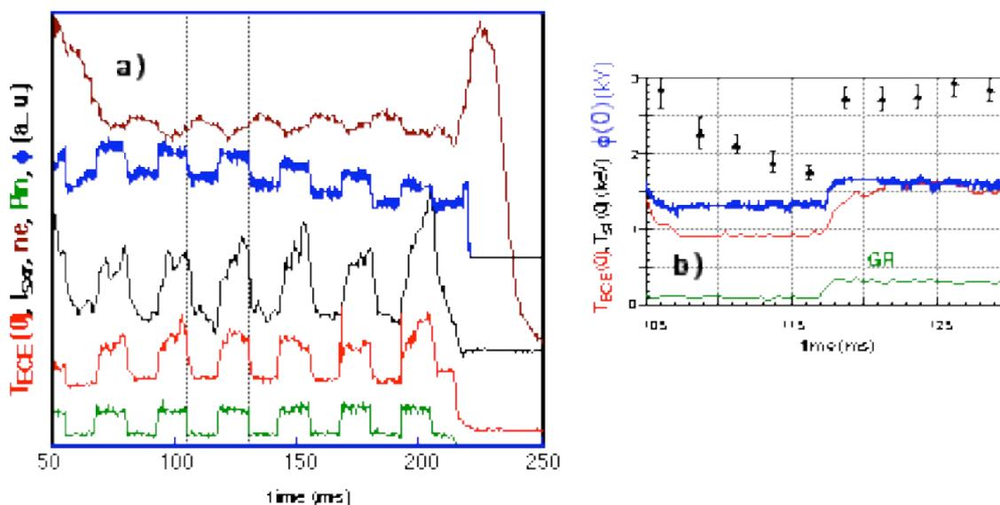
**Fig. 3.** Signals from an input power modulated discharge. a) temporal evolution of line density, central plasma potential, soft x rays intensity and central electron temperature. b) time evolution of characteristic suprathermal energy (black triangles).
