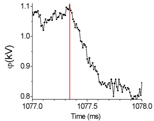
Fig.2. Time decay of plasma potential after ECRH (L2) is turned off.
