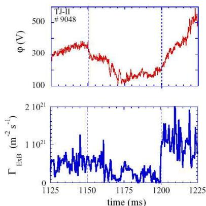
*Fig.6. Time evolution of edge plasma potential ( $\rho \sim 0.8$ ) measured by the HIBP system and the ExB turbulent transport measured by probes ( $\rho \sim 0.9$ ) during limiter biasing experiments ( $V_b = 200 \text{ V}$ ).*
