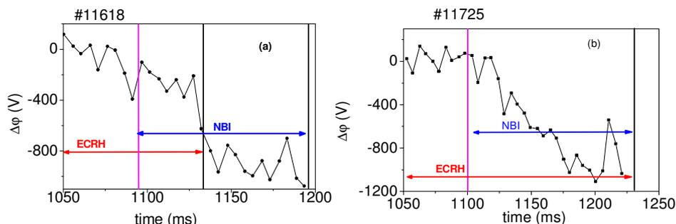
Fig 4: The time evolution of plasma potential during the transition from ECRH to NBI regimes.
