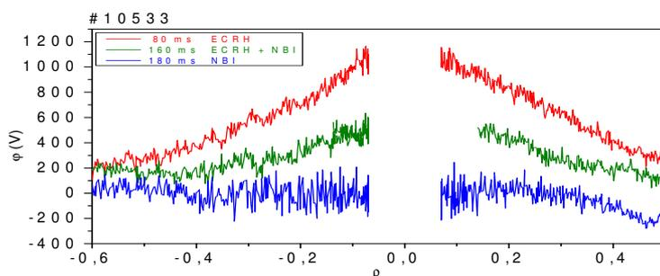
Fig.5: Radial profiles of plasma potential (ECRH + NBI)
