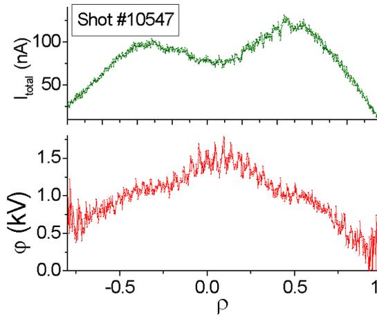
Fig.3. Influence of ECRH modulation ( 5 KHz ) on HIBP profiles.
