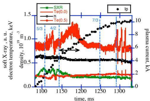
**Fig. 3. Same as Fig. 2 for a discharge with positive induction. From left to right, vertical dashed lines indicate the appearance of low order rationals –see labels- in the core. The last vertical line indicates the time at which  $u(0)/2\pi = 2.42$ .**
