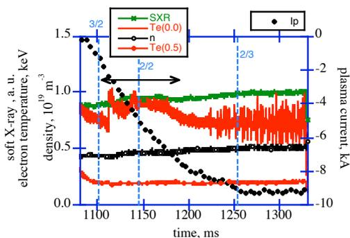
**Fig. 2. Time traces of soft X-ray emission from the plasma core (line with crosses), central  $T_e$  (line), line averaged density (line with dots),  $T_e$  at half minor radius (line with diamonds) and net plasma current for a discharge with negative induction.**
