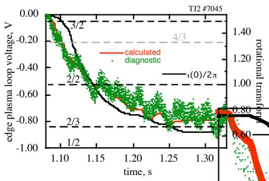
**Fig. 1. Comparison between calculated –at the plasma edge- loop voltage (light line) and loop voltage diagnostic (dots) for a discharge with induced ohmic current. The corresponding evolution of the magnetic axis rotational transform is drawn with a black line. Lowest order rational values within the range are shown with dashed lines.**
