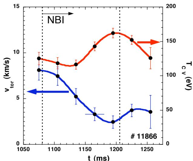
**Figure 3.** Temperature (eV) and toroidal rotation velocity behaviour from C V emission, with neutral beam injection heating (discharge #11866). The exposure time was 30 ms.
