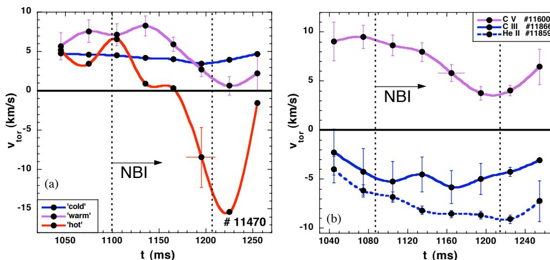
**Figure 2.** a) Toroidal rotation velocities from  $H_\alpha$  emission, with an exposure time of 30 ms. Discharge #11470. b) Toroidal rotation velocities from three impurities, C V ( $\rho \approx 0.5$ ), C III and He II (most external impurities), with 30 ms time resolution.
