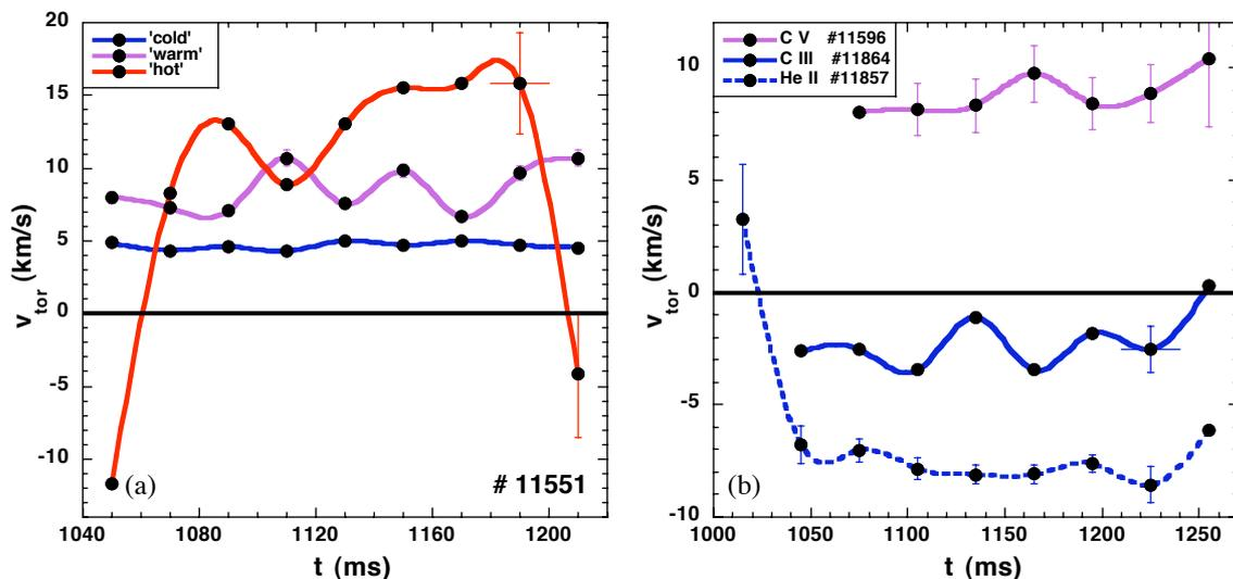
**Figure 1.** a) Toroidal rotation velocities from  $H_\alpha$  emission, with an exposure time of 20 ms. Discharge #11551. b) Toroidal rotation velocities for three impurities, C V ( $\rho \approx 0.5$ ), C III and He II (most external impurities), with exposure times of 30 ms. Positive values indicate co-magnetic field direction, negative values indicate counter-magnetic field direction.
