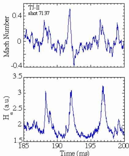
Fig. 2 Time evolution of parallel flows and edge instabilities in the boundary region of the TJ-II stellarator.
