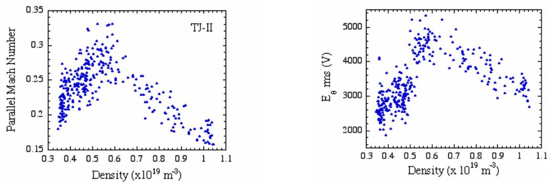
Fig. 3: Parallel flows and level of edge fluctuations versus plasma density in the plasma boundary of the TJ-II stellarator. Measurements were taken near  $\rho \approx 0.85$ .
