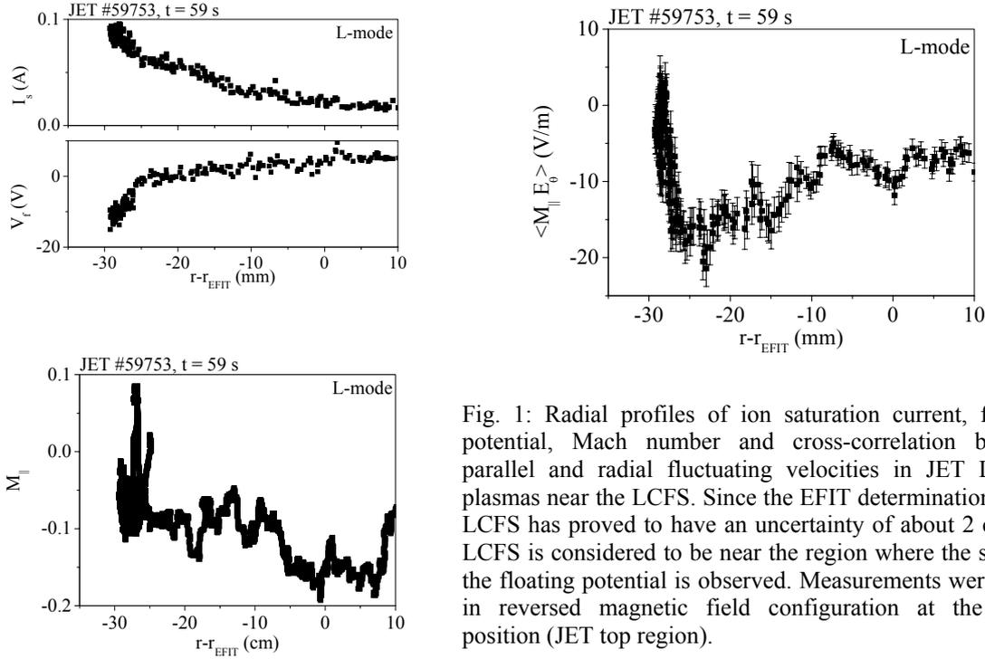
Fig. 1: Radial profiles of ion saturation current, floating potential, Mach number and cross-correlation between parallel and radial fluctuating velocities in JET L-mode plasmas near the LCFS. Since the EFIT determination of the LCFS has proved to have an uncertainty of about 2 cm, the LCFS is considered to be near the region where the shear in the floating potential is observed. Measurements were taken in reversed magnetic field configuration at the probe position (JET top region).
