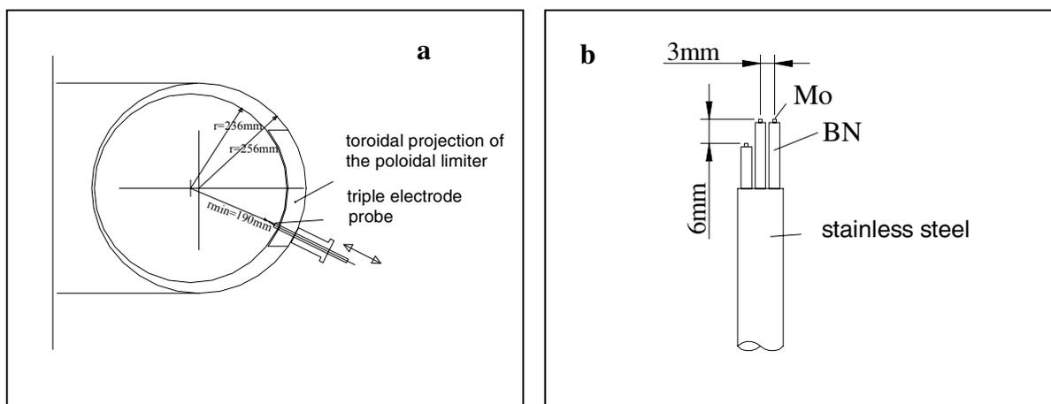
Figure 1. Experimental layout (a) and probe design (b).
