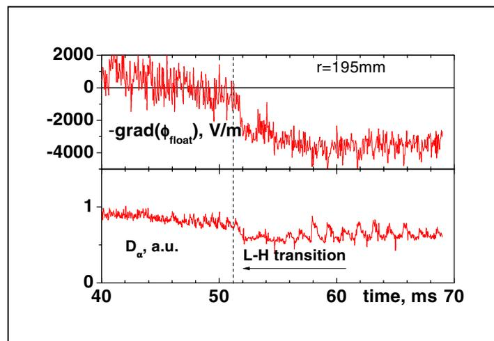
Figure 3. Temporal evolution of the floating potential during the ohmic L-H transition.
