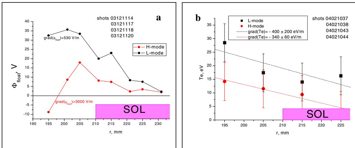
Figure 2. Spatial profiles of (a) floating potential and (b) electron temperature before (black) and after (red) ohmic L-H transition in the TUMAN-3M.
