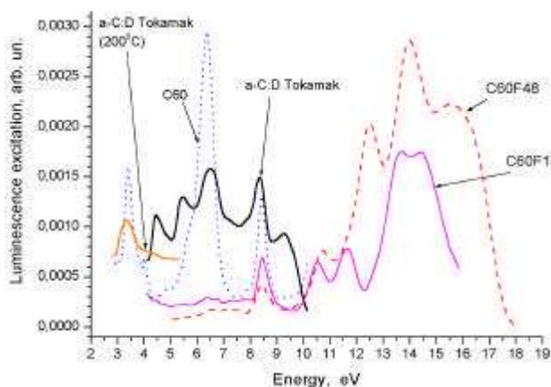
Fig.2. Films luminescence spectrum, excited by synchrotron radiation
