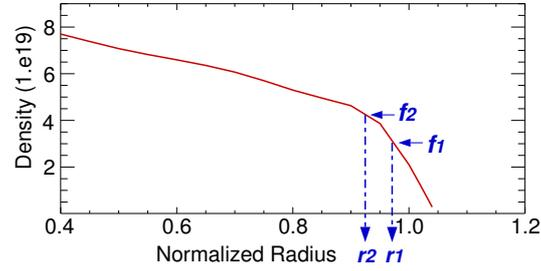
**Figure 1:** Density profile for an ELMy H-mode discharge (#17973,  $t = 6.03$  s).
