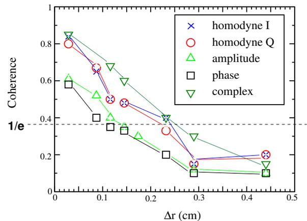
**Figure 4:** Coherence profiles measured during an L-mode discharge (#18761,  $k_{\perp} = 9.56 - 10.2 \text{ cm}^{-1}$ ).
