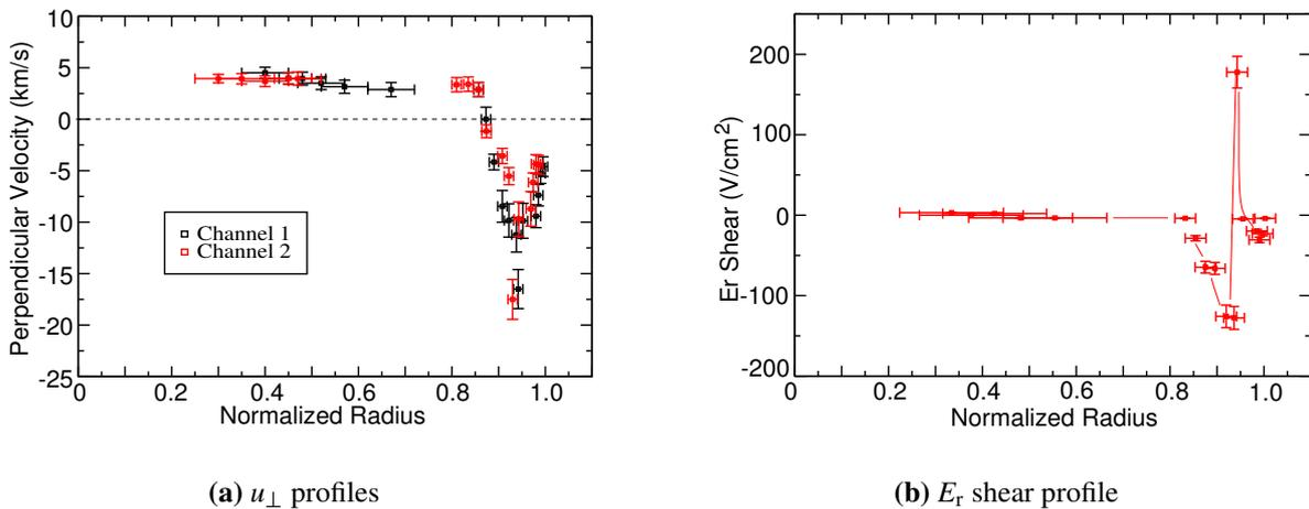
**Figure 2:**  $u_{\perp}$  profiles for two reflectometer channels from which the  $dE_r/dr$  is extracted for an H-mode discharge (#17973). The data was collected with both reflectometers in O-mode configuration.
