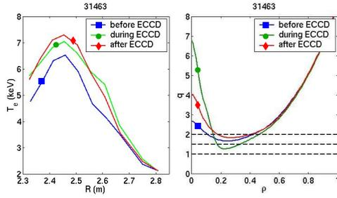
Fig. 2: electron temperature profiles (from ECE) versus major radius coordinate  $R$  and  $q$  profile (reconstructed by the CRONOS code) versus normalised radius, for discharge 31463.
