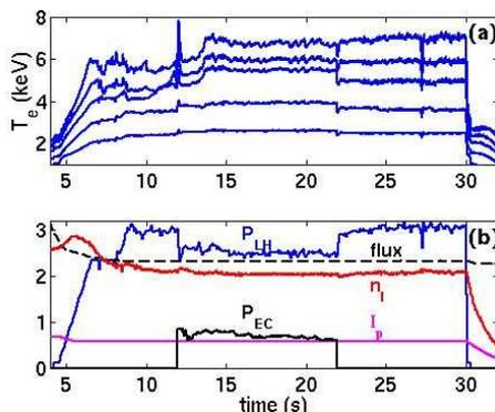
Fig. 1: Tore Supra discharge 31463. (a) Electron temperature measured by ECE at various plasma positions, covering the region  $0 \leq r/a \leq 0.4$ . (b) From top to bottom, as a function of time, LH power (MW), transformer flux (Wb), line integrated density ( $10^{19} \text{ m}^{-2}$ ), EC power (MW) and plasma current (MA).
