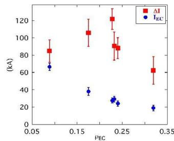
Fig. 5: Measured additional current driven by ECCD in the presence of LHCD (squares) and computed ECCD current (dots) versus the location (in normalized radius) of maximum EC power deposition (computed).
