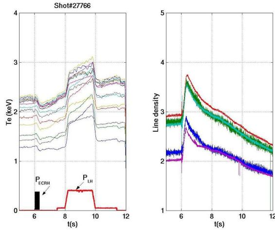
Fig. 3 Time evolution of the temperature (left) and the chord averaged density (right) during ECRH and LH power injection.
