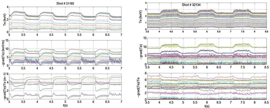
Fig.4 Time evolution of  $T_e$ ,  $-\nabla T_e$ ,  $-\nabla T_e/T_e$  during the ECRH power modulation experiment. Fig.5 Time evolution of  $T_e$ ,  $-\nabla T_e$ ,  $-\nabla T_e/T_e$  during the ICRH power modulation experiment.
