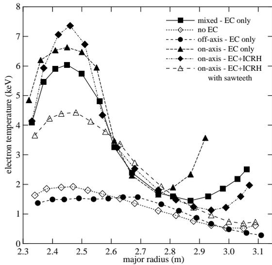
figure 2: electron temperature profiles, measured by ECE, for different ECCD scenarios
