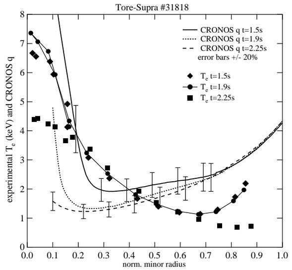
figure 4: measured electron temperature profiles and computed q profiles for a discharge with on-axis counter-ECCD and ICRH
