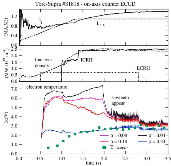
figure 1: time evolution of plasma parameters for a discharge with on-axis counter-ECCD and ICRH
