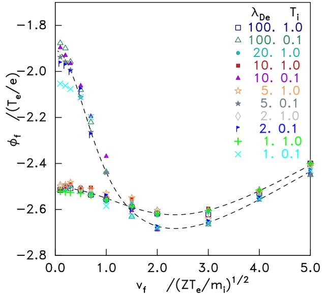
Figure 1: Floating potential calculated by SCEPTIC as a function of normalized drift velocity, for a range of  $\lambda_{De}$  measured in units of the sphere radius, and for  $T_i = 1$  and 0.1 times  $ZT_e$ . The dashed line shows the OML theory.
