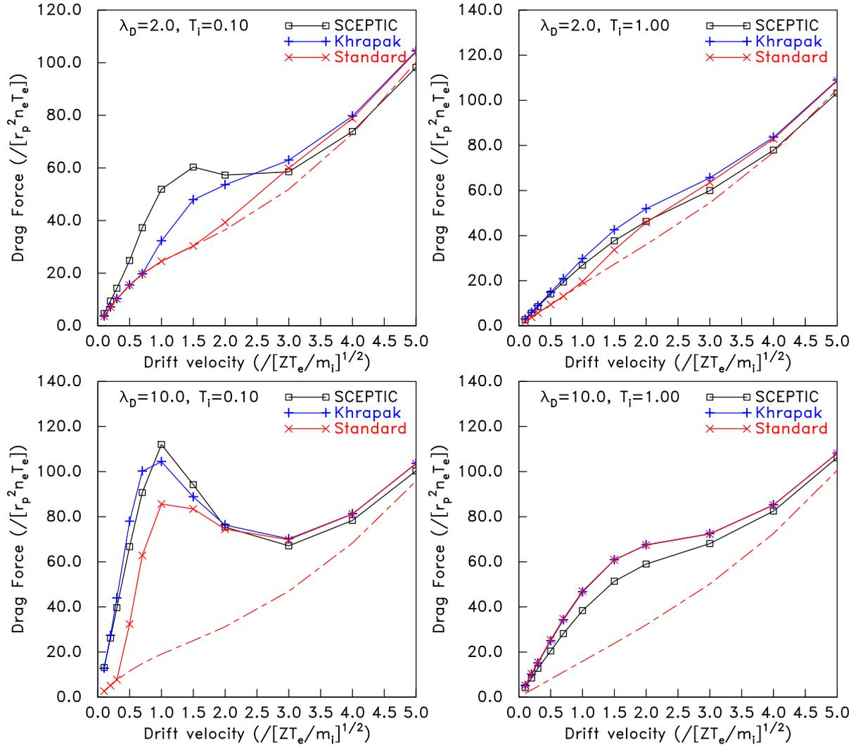
Figure 3: SCEPTIC calculations for  $\lambda_{De} = 2$  and  $10$ , on a computational domain of radius  $10$  and  $20$  respectively, times the probe radius; with  $T_i = 0.1$  and  $1.0 Z T_e$ .
