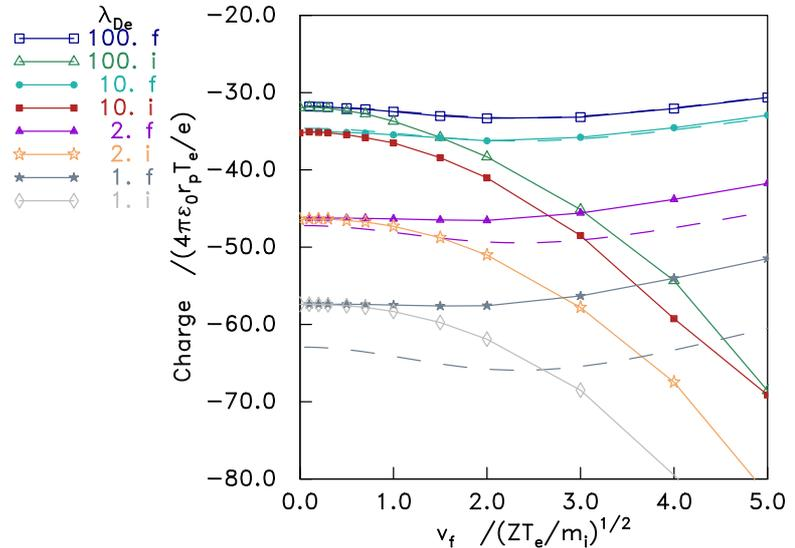
Figure 2: Charge as a function of drift velocity for an isolated sphere in a hydrogenic plasma ( $m_i = 1837m_e$ ,  $T_i = ZT_e$ ). A range of Debye lengths ( $\lambda_{De}$ ) is plotted, and both floating (f) and insulating (i) spheres. Dashed lines show the linearized-capacitance analytic approximation.
