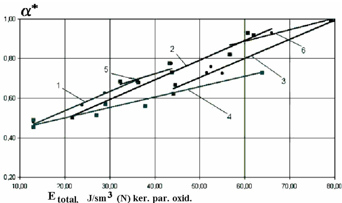
**Fig. 5.** Experimental dependencies relative degree of conversion of kerosine in syn-gas from total specific energy input in rezonator (cavity) plasmatron. 1,2,3- variable  $E_{\text{plasma}}$  at  $E_{\text{thermal}} = \text{const}$ ; 4,5,6- variable  $E_{\text{thermal}}$  at  $E_{\text{plasma}} = \text{const}$ .
