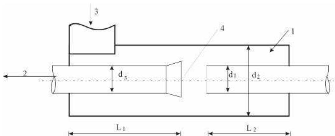
**Fig. 2.** Draft of construction scheme of resonator (cavity) microwave plasmatron.
