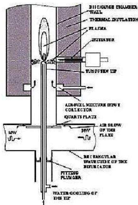
**Fig.1** Plasmachemical reactor with coaxial plasmatron.
