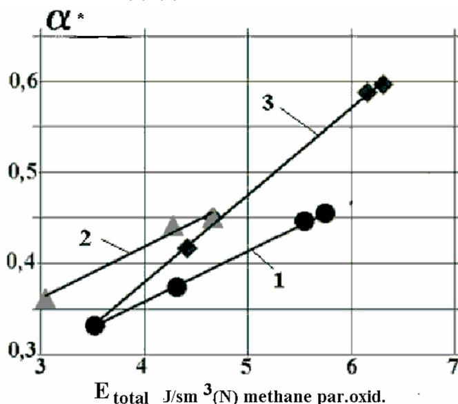
**Fig. 4.** Experimental dependencies relative degree of conversion of methane in syn-gas from total specific energy input in coaxial plasmatron. 1- variable  $E_{thermal}$  at  $E_{plasma} = 1.7 \text{ J/sm}^3 = \text{const}$ ; 2 – variable  $E_{thermal}$  at  $E_{plasma} = 3.0 \text{ J/sm}^3 = \text{const}$ ; 3- variable  $E_{plasma}$  at  $E_{thermal} = 1.7 \text{ J/sm}^3 = \text{const}$ ;
