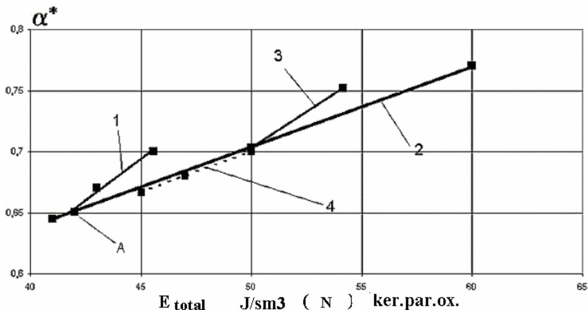
**Fig. 3.** Experimental dependencies relative degree of conversion of kerosene from total specific energy input in coaxial plasmatron. 1, 3 – variable only  $E_{plasma}$ ; 2 – variable only  $E_{comb}$ ; 4 – variable only  $E_{heat}$
