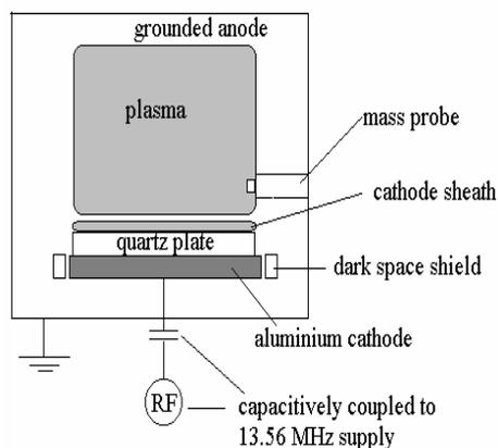
Fig. 1: A schematic diagram of the capacitively coupled discharge
