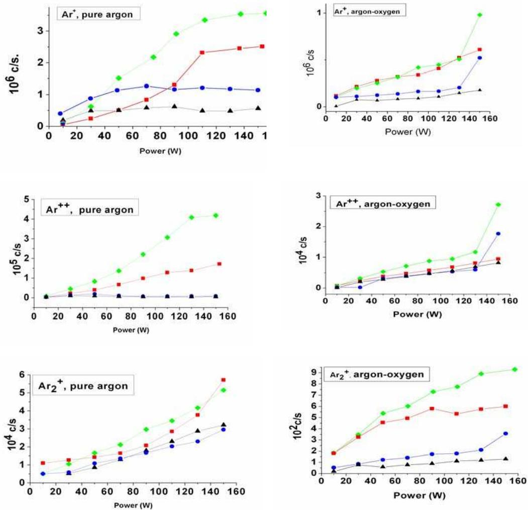
Fig. 3: Integrated intensities (fluxes of species) at different pressures: red for 20 mTorr, green for 40 mTorr, blue for 60 mTorr, black for 80 mTorr and different powers.
