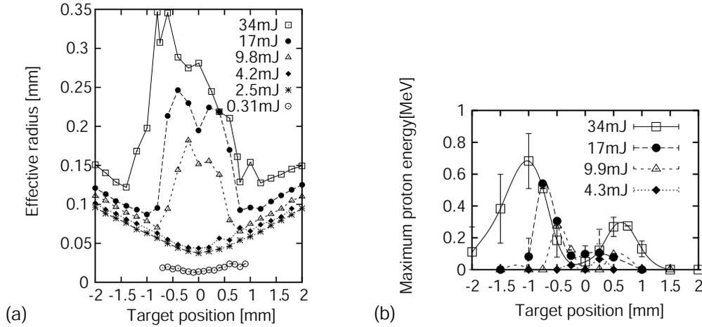
Figure 1: (a) Measured hole sizes as a function of the target positions at various laser energies. The vertical axis shows the effective radius defined by  $\sqrt{A/\pi}$ , where  $A$  is the measured area of a hole. The laser with an energy of 0.31 mJ penetrated the target only at a distance between -0.7 mm and 0.9 mm. (b) Dependence of maximum proton energies on target positions relative to the focal point observed on the forward side.
