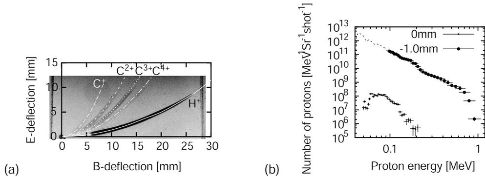
Figure 2: (a) Typical CR39 images of the Thomson parabola. The field strengths of the Thomson parabola were  $2.9 \times 10^5 \text{ V m}^{-1}$  electrically and 0.45 T magnetically. The laser energy was 34 mJ and the target position was -1.0 mm. The lines were calculated by MAFIA. Neutral particles were detected at the origin. (b) Energy spectra of protons at two target positions.
