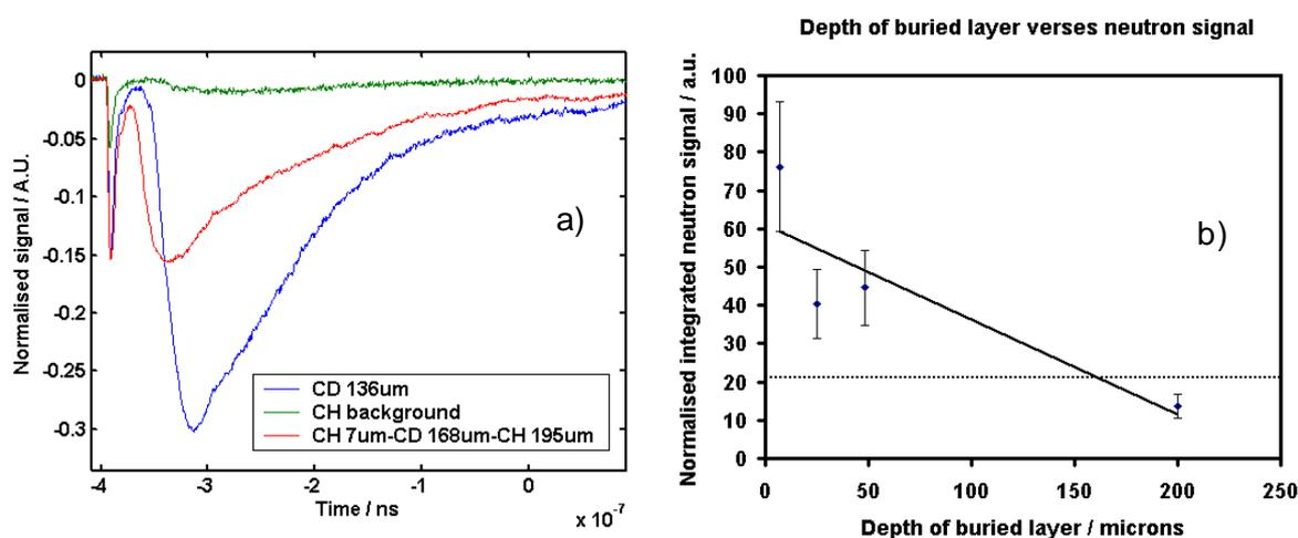
Figure 1 - a) Raw time of flight signals b) Plot of depth of buried layer against normalised, integrated signal, dotted line represents signal from plain CH targets.
