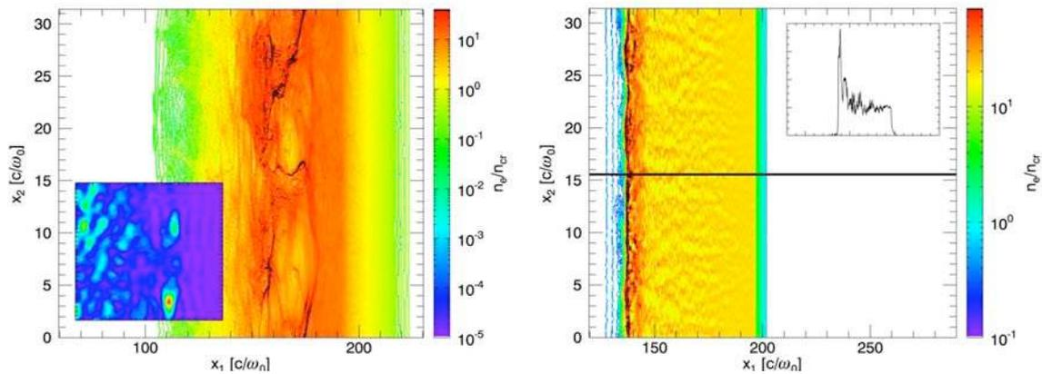
**Figure 3:** Electron density: low density target (left), and high density target (right). The inset shows the formation of photon bubbles (left), and the electron density along the axis (right)
