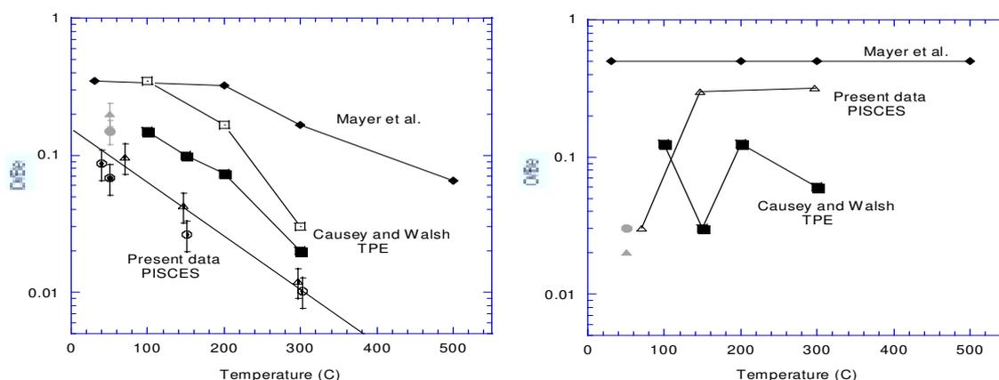
Figure 4 – D/Be and O/Be ratios for redeposited material collected on Ta (grey), Mo (dotted), and W (white) witness plate coupons as a function of collection temperature. Target temperatures are indicated by triangular (300°C) and circles (600°C).
