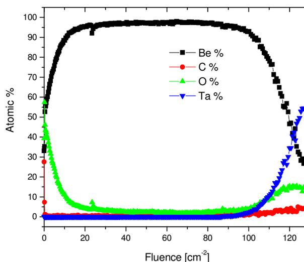
Figure 3 – Elemental depth profile of redeposited material collected during high-temperature exposure of a graphite sample to a beryllium containing deuterium plasma.
