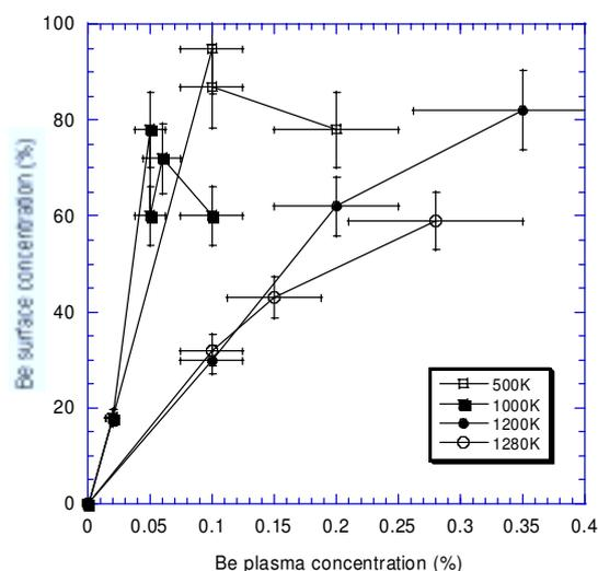
Figure 2 – Resulting equilibrium surface composition of graphite samples exposed to Be containing deuterium plasma.
